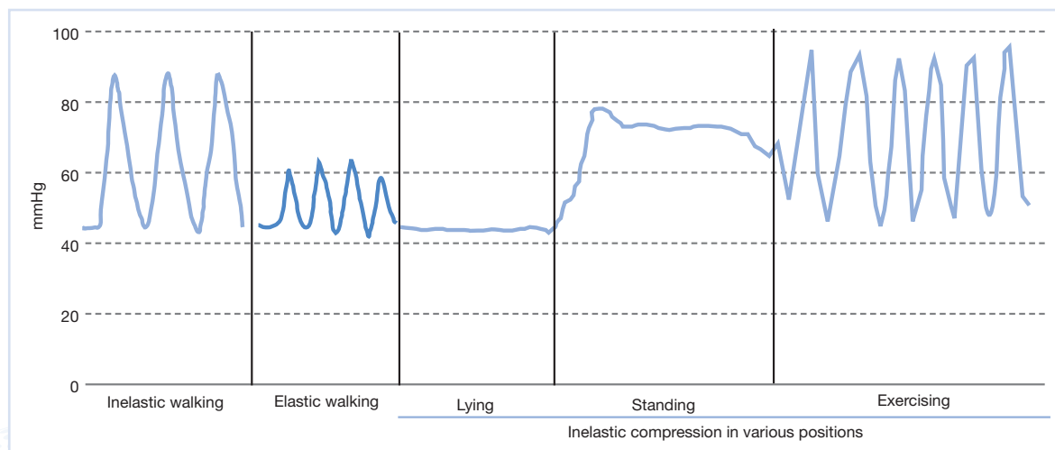
Fig 6. Graphic tracing of interface pressure measurements under inelastic and elastic compression with movement.
